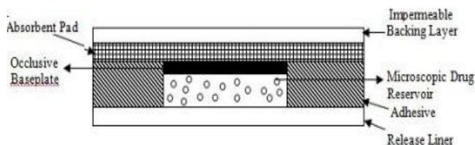
Fig. 3: Design of reservoir type transdermal patch [9]
