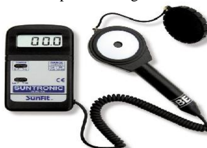
FIGURE 7: LUX METER FIGURE 8: UV METER CHARACTERISATION OF DEGRADANTS:
